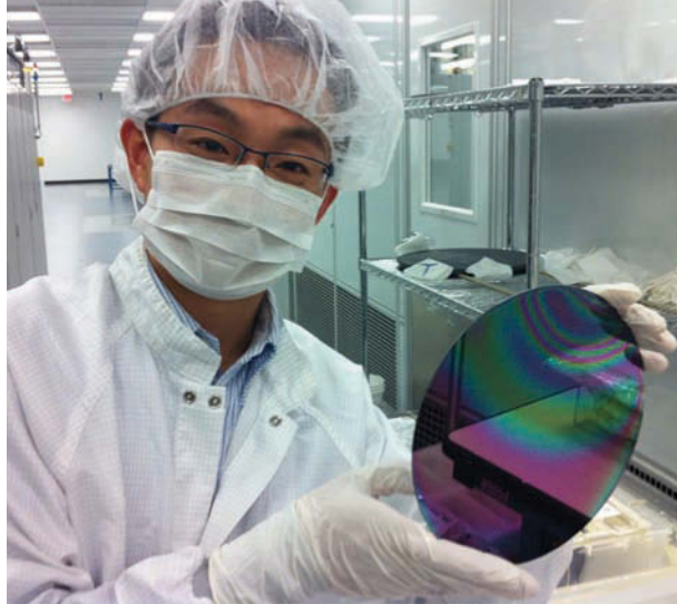
Bridgelux has demonstrated GaN-on-Si HB LEDs with performance comparable with that of LEDs employing SiC or ion-sapphire wafers, an advance that can ultimately result in lower-priced LED bulbs.
