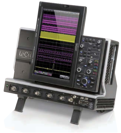
LeCroy's four-channel, 400- and 600-MHz-bandwidth WaveRunner 6 Zi HROs are unusual not only for their 12-bit ADC resolution but also for their pivoting displays. Another LeCroy family, the WaveMaster 8 Zi-A, uses patented digital bandwidth interleaving to achieve industry-leading 45-GHz bandwidth on one channel at 120G samples/sec. Bandwidth is 30 GHz/channel at 80G samples/sec on two channels and 20 GHz/channel at 40G samples/sec on all four channels.
