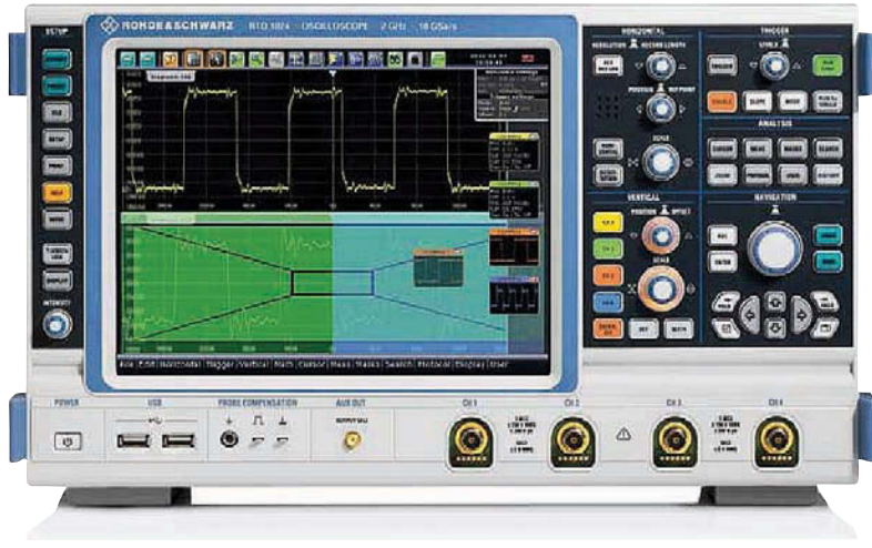
Rohde and Schwarz's RTO series includes a custom ASIC that enables the capture of more than 1 million waveforms/sec.
